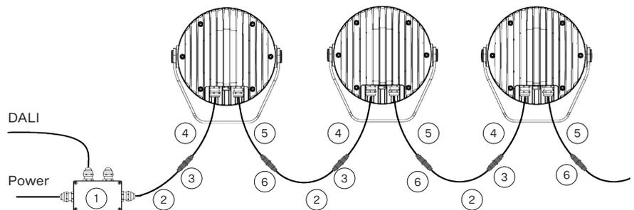
**Note: The last unplugged connector must be fitted with a Waterproof Cap to protect the IP rating.**
