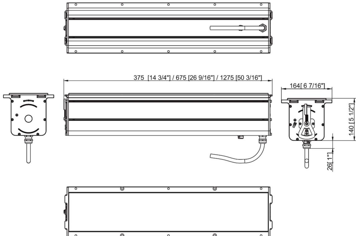
**Dimensions with mounting sleeve (All dimensions in mm [inch])**
