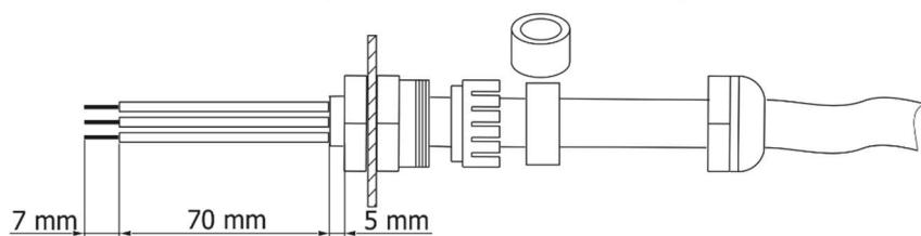
**Reducing seal** (P/N 13051388) - enclosed, standard seal has to be removed before installing this seal
