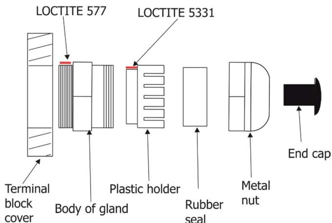
The cable gland M20 MS with a standard seal serves for a cable of diameter of 7-13mm, for smaller diameter of cable (4-8mm) you have to remove the original seal from the cable gland M20 and use the enclosed reducing seal instead of it. The reducing seal for diameter of cable 4-8mm (P/N 13051388) is enclosed in the Booster box.
