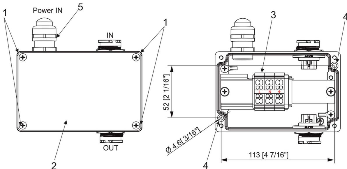
The Cable gland M20x1.5 for Power IN (5) is intended for a cable of a diameter of 7-13mm. Remove the end cap from the cable gland before passing the cable.
