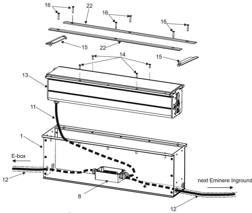
The supply/data cable to and from the mounting sleeve must be placed in a protective tube (12).
