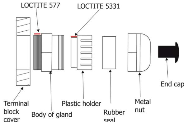
We recommend to apply an adequate layer of the paste LOCTITE 5331 on the plastic holder of the cable gland before inserting it into the body of the gland and an adequate layer of the paste LOCTITE 577 on the thread of the gland body in case that you need to unscrew and remove the cable gland from the housing of the junction box and and screw it back to the housing.
