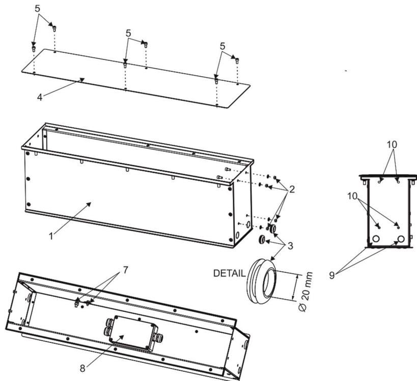
5. Connect the Eminere Inground MC (13) and all needed cables to the junction box (8).
