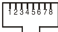
RJ-45 socket (front view):
