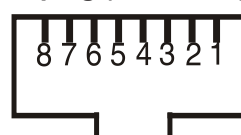
RJ-45 plug (front view):
