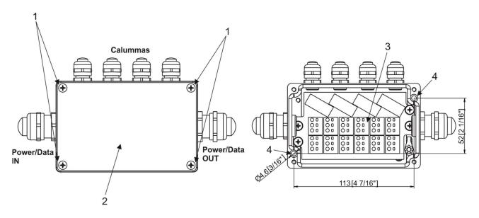
1. Unscrew the four screws (1) from the cover (2) on the junction box to get access to the PCB with terminal
