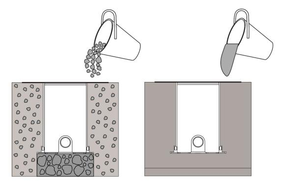
Note: the Lyrae XS FIX can be installed with the Bevel Edge Trim or the Flush Trim. Every trim version requires different height of filling material on the top edge of the mounting sleeve:
