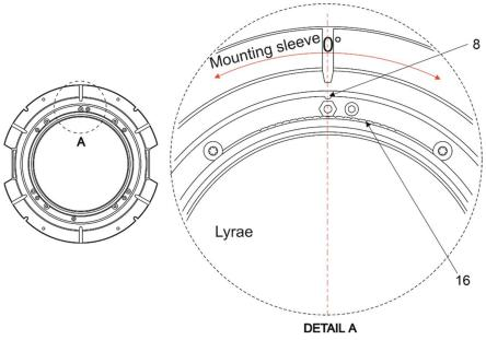
**12.** Fasten the Lyrae M to the mounting sleeve by means of the four Allen screws M6x20 (17). Place the trim (19) on the Lyrae M and fasten it by means of three flat Allen screws M6x35 (20).
