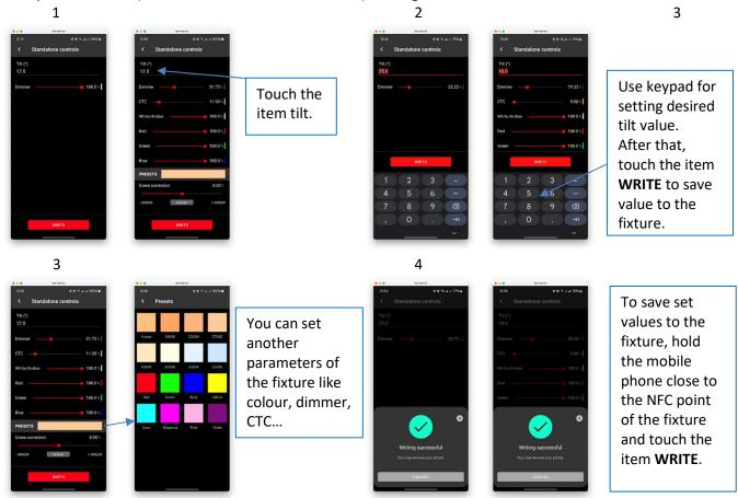
Movement of the light beam is approximately 2-3 seconds delayed after writing a tilt value to the Lyrae S. The tilt setting by NFC is disabled. If the Lyrae S is set to DMX mode 10.
