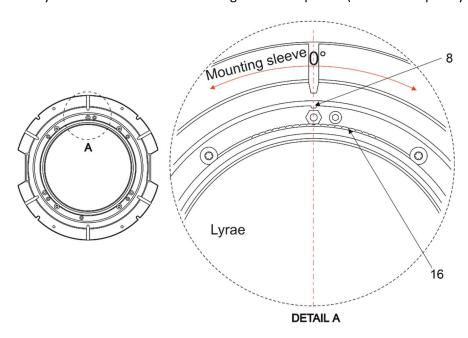
**3.** Fasten the mounting sleeve to the bottom of the mounting hole by means of four apertures (9) with diameter of 5.3 mm. Use fasteners suitable for your mounting surface.
