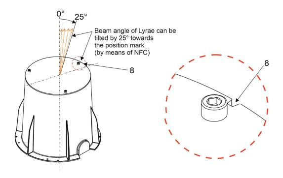
Detail of the Lyrae M inserted in the mounting sleeve – top view (without temporary cover):
