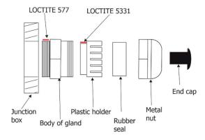
Failure to properly install cable glands will result in failure of the watertight seal!
