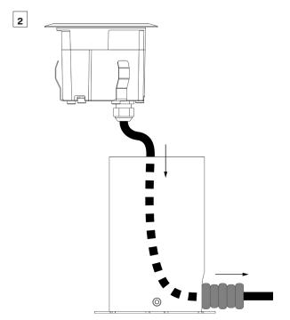
Insert the cable from the Luminaire into the Sleeve and pull it through the conduit.
