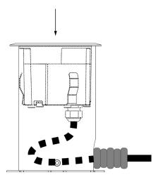
Insert the Luminaire into the Sleeve.
