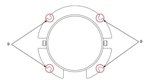
5. The mounting hole can be filled up with soil, gravel or concrete. Filling material should be in the same level with the top of the temporary cover (for Flush Trim) or with the top edge of the mounting sleeve (for Bevel Edge Trim).
