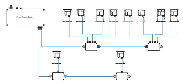
NOTE: NOTE: DMX data line of Lyraes XS FIX at each LED output of the E-box has to be terminated at the last fixture.
