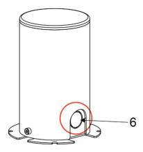
2. Insert the mounting sleeve into the mounting hole and level it using a spirit level (7).
