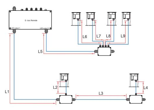
Total cable length=L1+L2+L3+L4+L5+L6+L7+L8+L9
