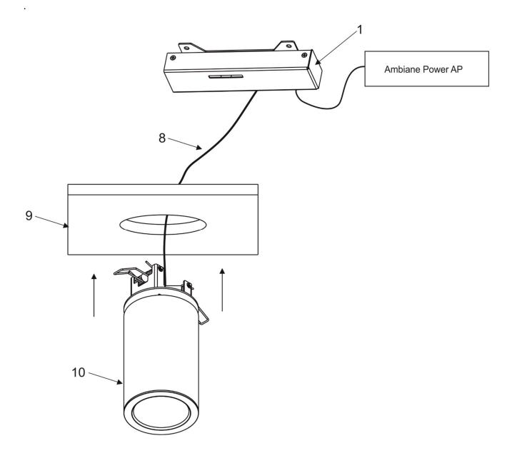
9. Secure the LED unit (10) in desired position by means of two spring clips (11).
