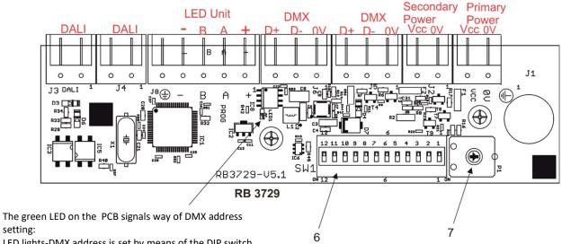
setting: LED lights-DMX address is set by means of the DIP switch. LED does not light- DMX address is set by means of RDM.
