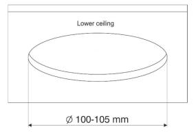
**2.** Place the control unit (1) above the ceiling through the ceiling opening and fasten it by means of two holes in the housing of the control unit and suitable fasteners.
