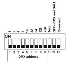
DIP 10 - if it is switched to ON=test light, the fixture lights at 3200K (for RGBW and TW version) DIP 11 - has to be switched to OFF position to receive DMX 512 and DALI, position ON=0-10V control
