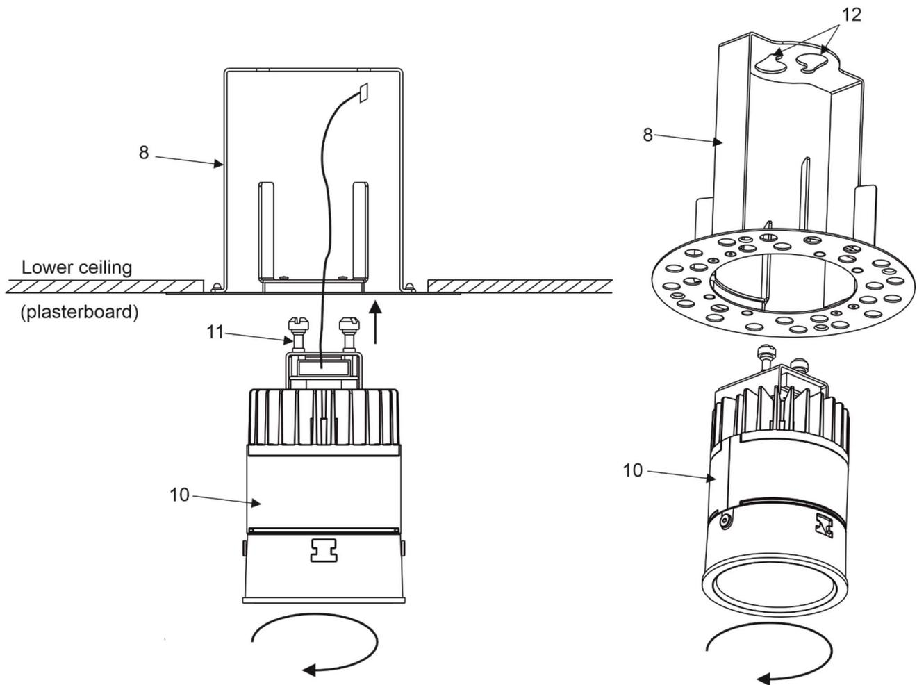
Note. For inserting the LED unit (10) to the mounting bracket (8) use the suction cup (optional part).
