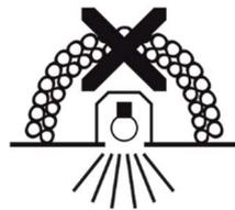
Unsuitable for covering by heat insulation material
