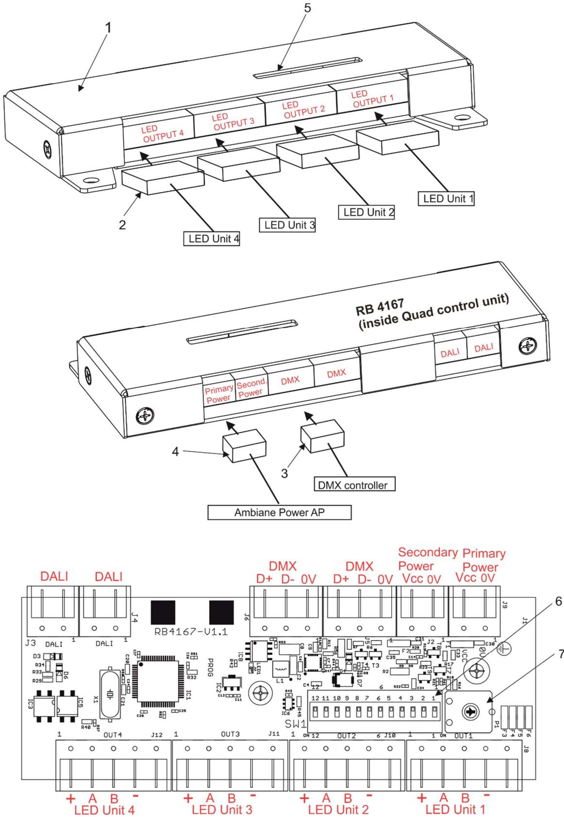
The DIP switch (6) is accessible by the aperture (5) in the cover of the control unit (1).
