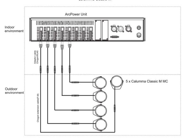
Fixture's Chogori connector is water protected according to IP 67 by mating with related Chogori connector. It cannot stay disconnected outdoor without covering the waterproof cap (optional item).
