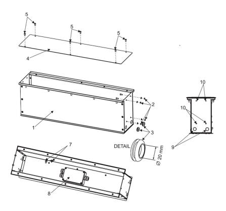
**5.** Connect the Eminere Inground (13) and all needed cables to the junction box (8). Note: the cabel (11) of the Eminere Inground is 2 m long, we recommend to shorten the cable on 1 m.
