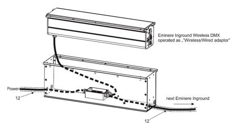
The supply cable to the mounting sleeve and power/data cable from the mounting sleeve must be placed in a protective tube (12).
