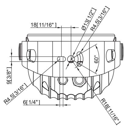
The LED module (4) can be tilted +180°/-180°. Use an Allen key 2.5 for adjusting a LED module position.
