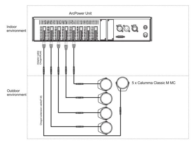
Fixture's Chogori connector is water protected according to IP 67 by mating with related Chogori connector. It cannot stay disconnected outdoor without covering the waterproof cap (optional item).
