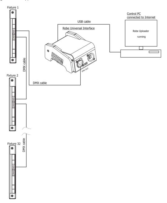
The fixtures have to be connected in a daisy-chain (max. 32 fixtures) and via the Robe Universal Interface/Robe Universal Interface WTX and a USB cable connected to the control PC with the Robe Uploader running. The fixtures have to be connected to power. The control PC should be connected to the Internet.
