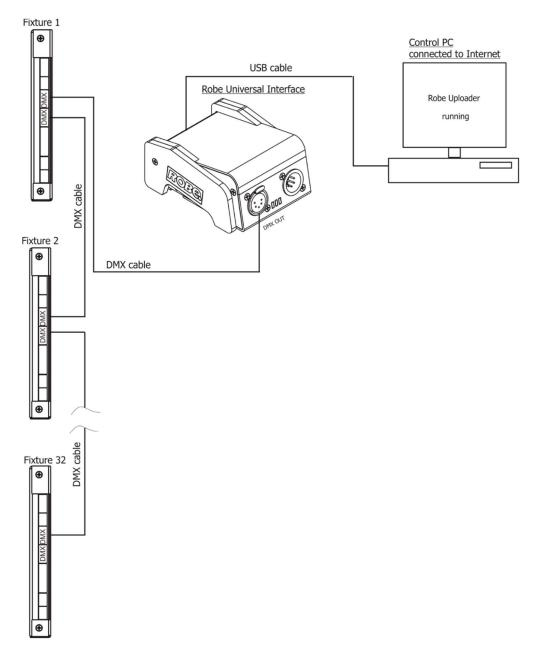
The fixtures have to be connected in a daisy-chain (max. 32 fixtures) and via the Robe Universal Interface/Robe Universal Interface WTX and a USB cable connected to the control PC with the Robe Uploader running. The fixtures have to be connected to power. The control PC should be connected to the Internet.
