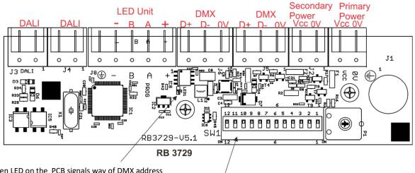
The green LED on the PCB signals way of DMX address setting:
