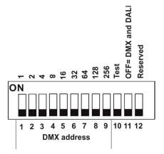
DIP 10 - if it is switched to ON=test light (the fixture lights at 3200K (for RGBW and TW version)) DIP 11 - has to be switched to OFF position to receive DMX 512 and DALI, position ON=0-10V control
