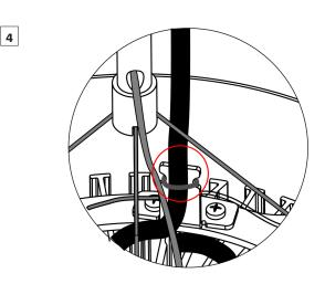
Fasten the LED unit's cable to holder using a cable binder.
