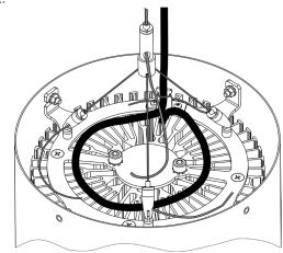
Store an redundant cable as instructed on the picture above. Maximum of one full loop to prevent overheating.
