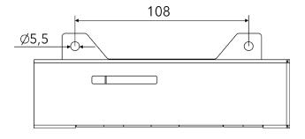
Fasten the control unit on the ceiling by means of two holes in the control units housing.
