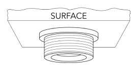
Fasten the Ceiling Plate M6i to the lower ceiling with suitable fastener.
