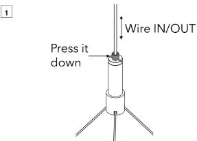
Press down the pin on the wires connector for length adjustment.
