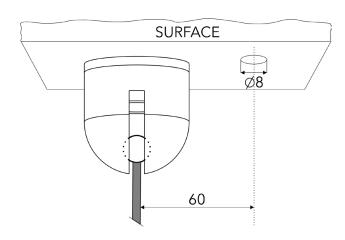
Drill the hole Ø8mm in the lower ceiling for the LED unit supply cable. If you wish to have the LED unit supply cable parallel with the hanging wire, the distance between the hanging wire and the LED unit supply cable should be 60mm.
