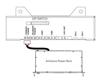
Install terminal block to power cable (from Ambiane Power Rack or Ambiane Power XP) and connect it to Primary power socket of the control unit.
