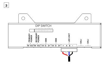
Install terminal block on LED unit's cable and connect it to the control unit.
