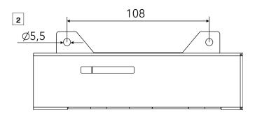
Mount the control unit to ceiling via two mounting holes and suitable fasteners.
