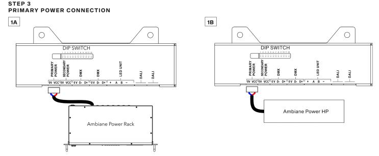
Install terminal block to power cable (from Ambiane Power Rack or Ambiane Power HP) and connect it to Primary power socket of the control unit.
