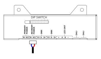
Install terminal block on Secondary power cable and connect it to Secondary power socket of the control unit.
