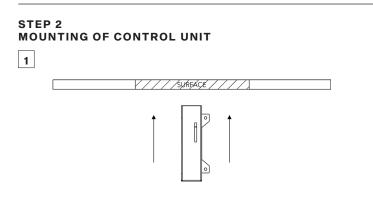
Place control unit above the ceiling through the ceiling opening.
