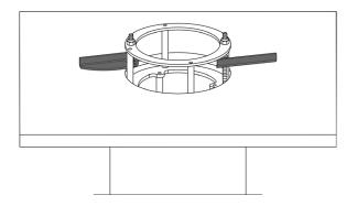
Tighten the holders on both sides until the fixture is firmly secured to the ceiling.
