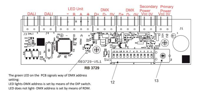
Note: The trimmer (13) allows you to set a light intensity (for secondary power only). This trimmer is accessible by aperture (18) in the cover of the control unit (1).
