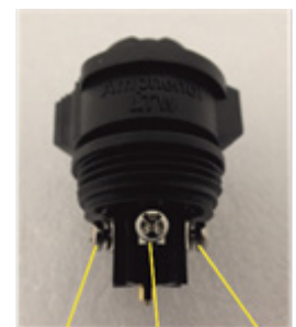
D- Orange wire 0V Shielding D+ Red wire N White wire Earth Green wire L Black wire
