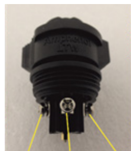
D+ Red wire 0V Shielding D- Orange wire L Black wire Earth Green wire N White wire
