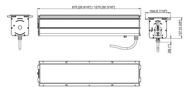
Dimensions with mounting sleeve (All dimensions in mm [inch])
