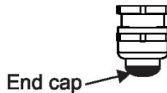
5. Pass cable for DMX through cable glands M12x1.5 and connect it to the terminal block and tighten the cable in the cable gland.
