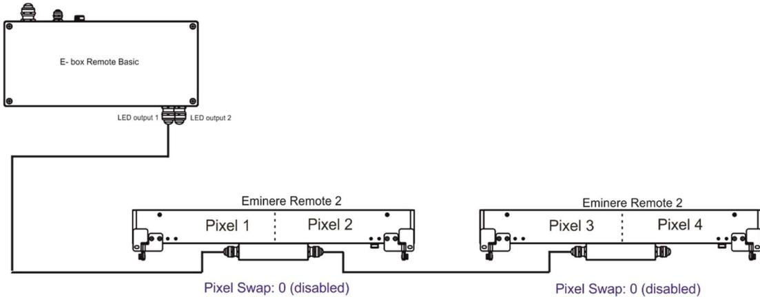
In case of reconnecting the E-box Remote Basic on the other end of Emineres Remote line, the pixel order is not in succession:
