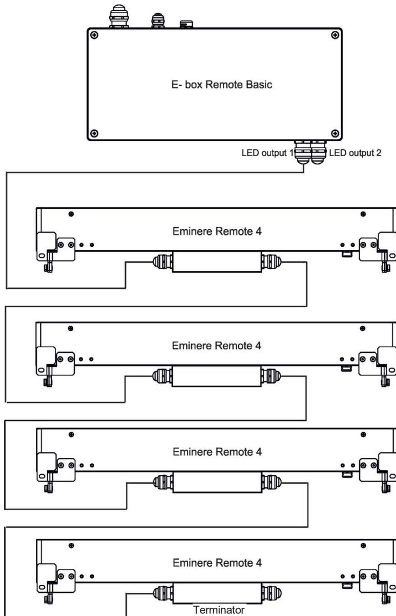
Each line of Emineres Remote connected to the LED output of the E-box Remote Basic has to be terminated at the last fixture.
