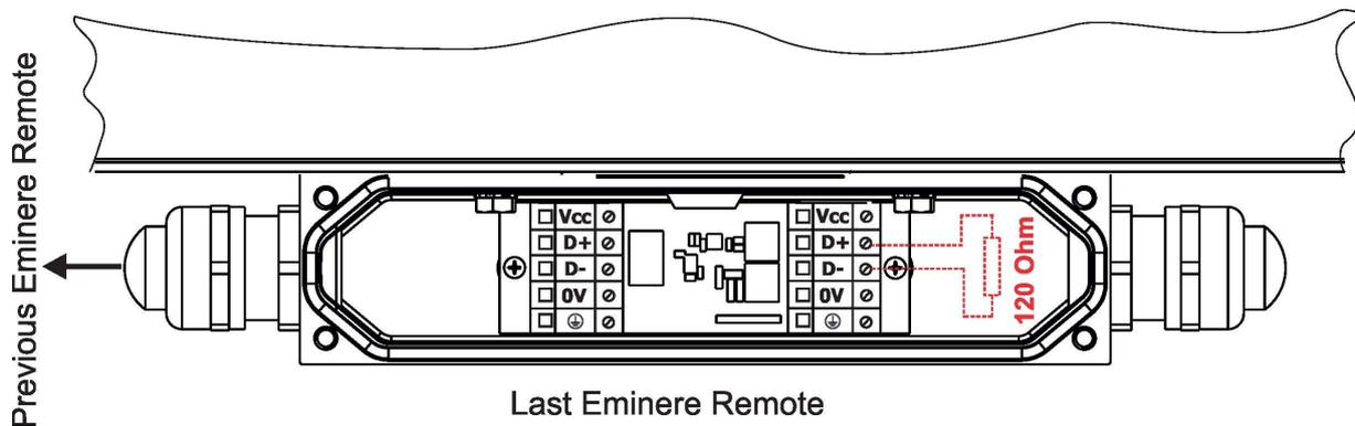
The number of Emineres Remote connected to one LED output of the E-box Remote Basic depends on the type of Eminere Remote and cable length.
