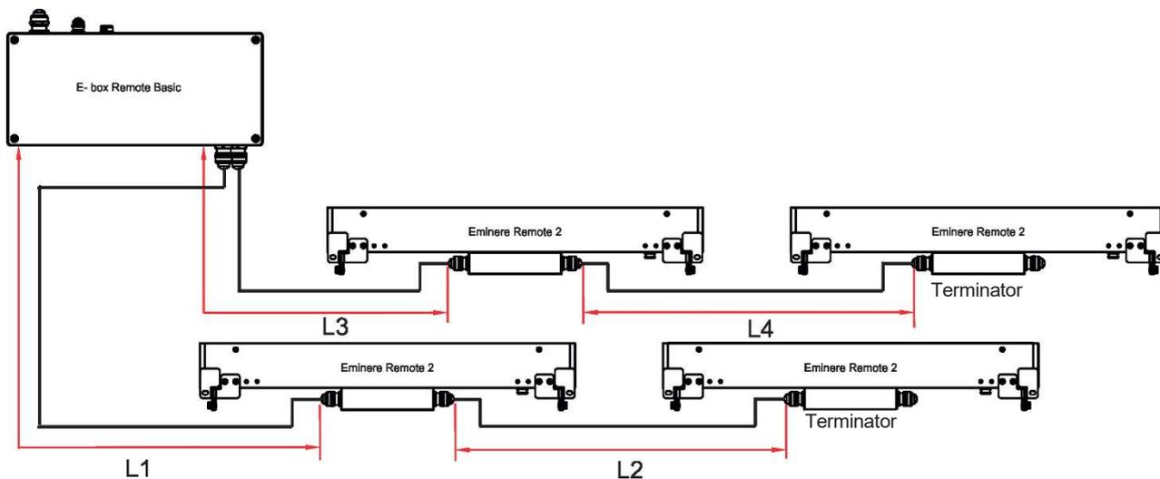
Max. number of Eminere Remote modules connected to the one output of the E-box Remote Basic is stated in the following table.
