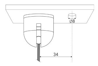
Drill the hole Ø8mm in the lower ceiling for the LED unit supply cable. If you wish to have the LED unit supply cable parallel with the hanging wire, the distance between the hanging wire and the LED unit supply cable should be 60mm.
