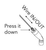
Press down pins on the hanging wires anchors for length and downward orientation adjustment.
