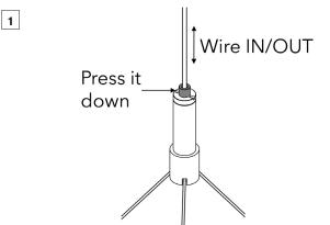
Press down the pin on the wires connector for length adjustment.
