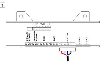
Pull the LED unit's cable through prepared hole in the ceiling and secure it above ceiling. Install a terminal block on the cable and connect it to the control unit.
