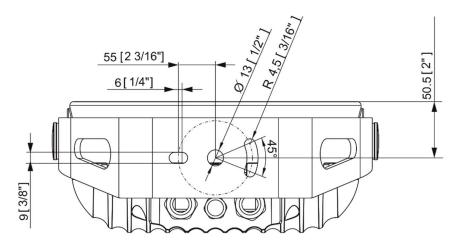
The LED module (4) can be tilted +180°/-180°. Use an Allen key 2.5 for adjusting a LED module position.
