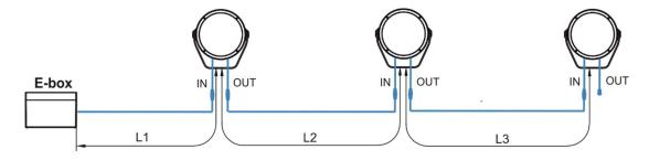
**Notice for the E-box Star**: The tables above state max. total number of Calummas connected to 6 LED outputs of the E-box Star (or max. number of Calummas connected to one output if the rest of outputs is not connected).
