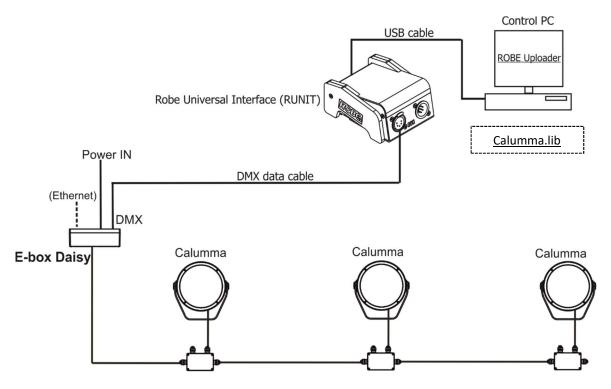
If you use a connection via junction boxes and you need to update connected E-box, switch the E-box to the Standard mode and use the <a href="EminereEbox.lib">EminereEbox.lib</a> in the ROBE Uploader to update E-box. After updating the E-box, switch it back to the Pass-Trough mode.
