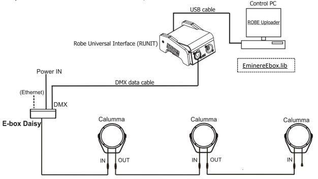
2. By means of the Ethernet connection. IN/OUT connection.
