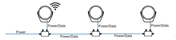
**Note:** This type of connection must have M, L or XL versions as the first luminaire. Next luminaires in a row could be chosen from S, M, L or XL versions.
