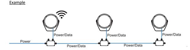
**Note:** This type of connection must have M, L or XL versions as the first luminaire. Next luminaires in a row could be chosen from S, M, L or XL versions.
