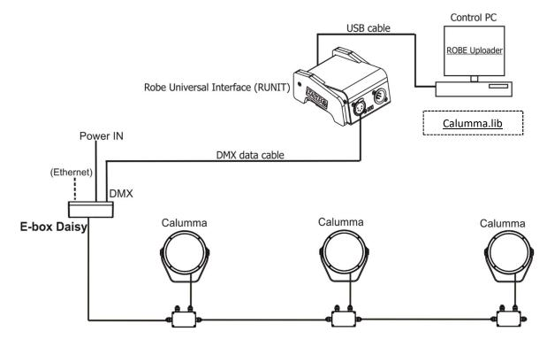
If you use a connection via junction boxes and you need to update connected E-box, switch the E-box to the Standard mode and use the <u>EminereEbox.lib</u> in the ROBE Uploader to update E-box. After updating the E-box, switch it back to the Pass-Trough mode.
