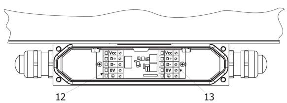
Wiring of connection blocks (12,13) in the junction box.
