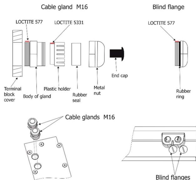
5. Pass the power/data cable through one cable gland (4) and connect to the terminal block.
