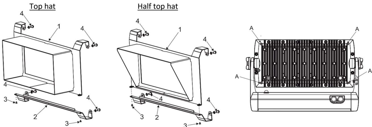
6. Unscrew screws M3x5 (3) to remove the bottom part (2) of the top hat (half top hat).
