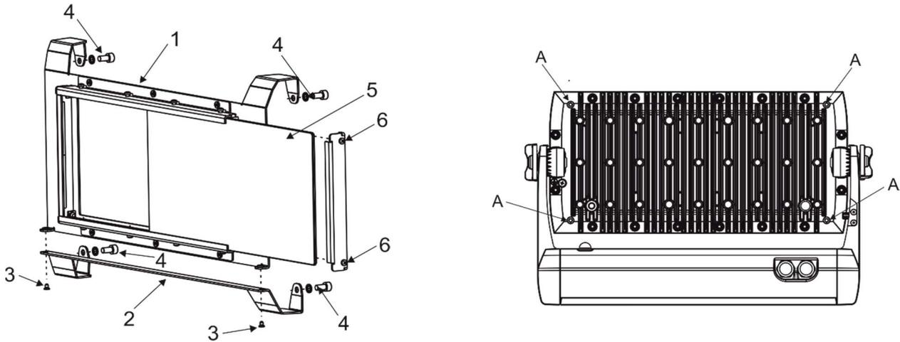
1. Unscrew two screws M3x5 (3) to remove the bottom part (2) of the adaptor black glass.
