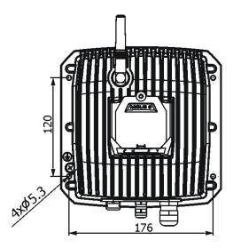
Four holes with diameter of 5.3mm in the control unit are intended for mounting on a flat, non-flammable surface. The length of the connection cable between the ArcPower 48 Outdoor and the LED unit should not exceed 20 m (at 700mA load) or 80m (at 350mA load).
