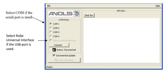
If the connection is OK, click on the Start Uploading button to start uploading. It will take several minutes to perform software update. If the option "Incremental Update" is not checked, all processors will be updated (including processors with the same software version).
