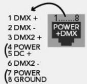
**CHECK PIN CONFIGURATIONS. APPLYING POWER TO THE DMX INPUT WILL DAMAGE THE CONTROLLER. MAKE SURE THE CONTROLLER IS MOUNTED WITHOUT TOO MUCH FORCE BEHIND AS THIS CAN PUSH APART THE GLASS.**
