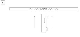
Place control unit above the ceiling through the ceiling opening.
