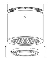
Tighten the holders on both sides until the fixture is firmly secured to the ceiling.
