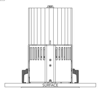
Holders in extended downward position holding the fixture in the ceiling opening.
