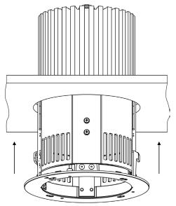
Insert luminaire into prepared ceiling opening.
