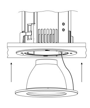
Insert Top frame with optics into luminaire.
