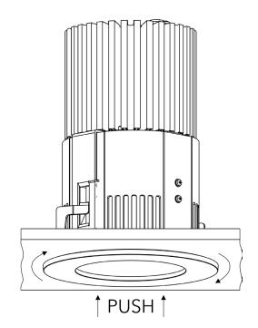
Push Top frame into luminare and twist it clockwise, until it's locked in the position.
