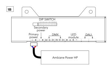
Install terminal block to power cable (from Ambiane Power Rack or Ambiane Power HP) and connect it to Primary power socket of the control unit.
