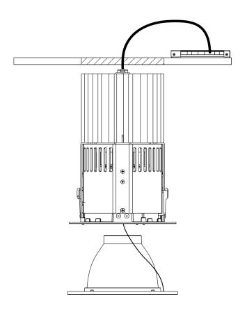
LED unit connected to control unit prior to mounting.
