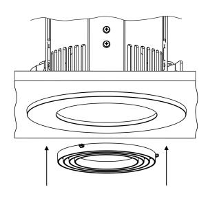
Insert the Ring Louver into the Top frame.
