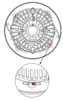
Locks that are holding a Front frame of luminaire.
