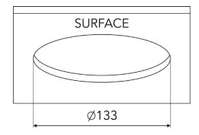
Standard mounting hole with diameter of 133mm.
