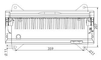
Drill holes to the surface according to holes spacing. Mount Divine via mounting holes on the surface.
