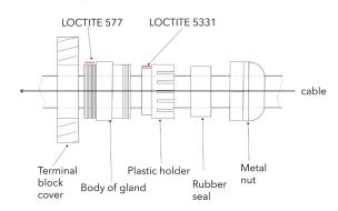
We recommend to apply an adequate layer of the paste LOCTITE 5331 on the plastic holder of the cable gland before inserting in into the body of the gland and an adequate layer of the paste LOCTITE 577 on the thread of the gland body.
