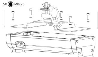
Mount the adaptor using 5 screws.
