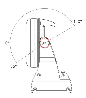
Release locking screw on each sides. Angle fixture to desired position and tighten locking screw on each sides.
