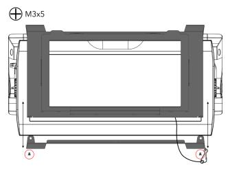
Unscrew two screws and split accessory to two parts. Place each part onto the luminaire's head and screw them together.
