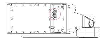
Inlets for power and data from bottom side of the luminaire.
