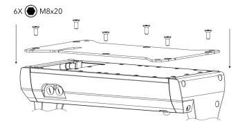
Mount the adaptor using 6 mounting screws.
