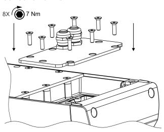
Before applying the torque, make sure the thread is clean and functional.
