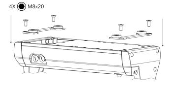
Mount pair of rubber feet using 4 screws.
