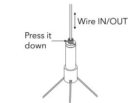
Press down the pin on the wires connector for length adjustment.
