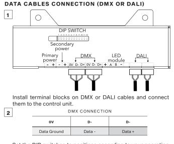
Set the DIP switches to positions according to your operation mode. The fixture can be controlled by DMX or DALI (switch 11 in OFF position).
