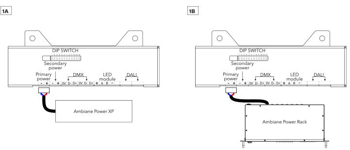
Install terminal block to power cable (from Ambiane Power Rack or Ambiane Power XP) and connect it to Primary power socket of the control unit.
