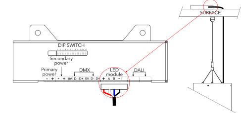
Pull the LED unit's cable through prepared hole in the ceiling and secure it above ceiling. Install a terminal block on the cable and connect it to the control unit.
