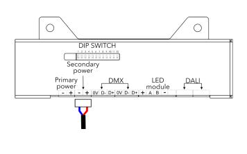
Install terminal block on Secondary power cable and connect it to Secondary power socket of the control unit.
