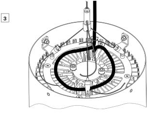
Store an redundant cable as instructed on the picture above. Maximum of one full loop to prevent overheating.
