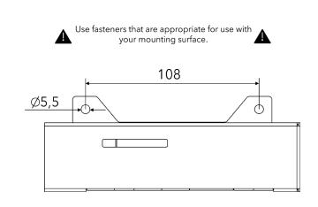
Fasten the control unit on the ceiling by means of two holes in the control units housing.
