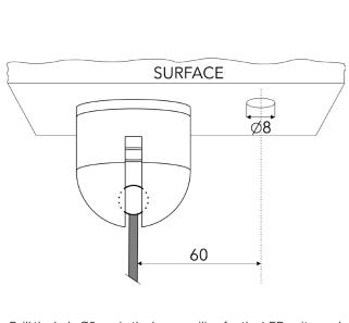
Drill the hole Ø8mm in the lower ceiling for the LED unit supply cable. If you wish to have the LED unit supply cable parallel with the hanging wire, the distance between the hanging wire and the LED unit supply cable should be 60mm.
