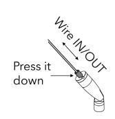
Press down pins on the hanging wires anchors for length and downward orientation adjustment.
