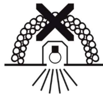
Unsuitable for covering by heat insulation material
