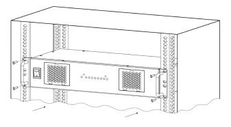
Fasten the Ambiane Power Rack into rack by means of two screws on each side of the Ambiane Power Rack .
