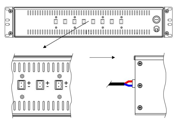
Install a terminal block on power cable and connect it to the Ambiane Power Rack.
