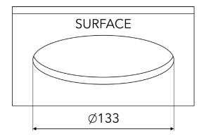
Prepare cut-out with diameter of 133 mm.
