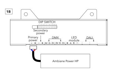
Install terminal blocks to power cables and connect them in to primary power socket of the control unit.
