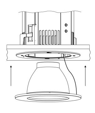
Insert Top frame with optics into luminaire.
