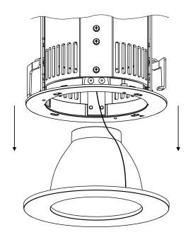
Push in and twist the Front frame counter-clockwise to release it from locks.
