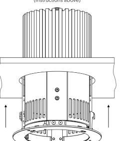
Insert luminaire into ceiling opening.
