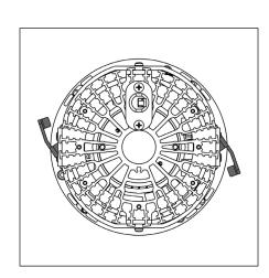
Top view of luminaire with extended holders.
