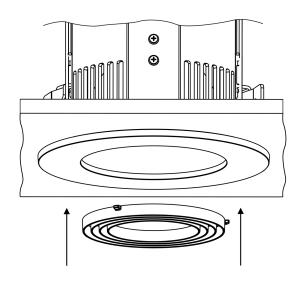
Insert the Ring Louver into the Top frame.
