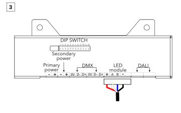
Install terminal block on LED module's cable and connect it to the control unit.
