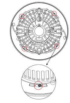
Locks that are holding a Front frame of luminaire.
