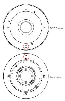
Position the Top frame according to installation marks. Marks of the luminaire and Top frame must be on top of each other.
