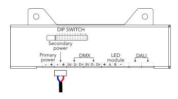
Install terminal block on power cables and connect them to Secondary power socket of the control unit.
