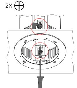
Secure the luminaire in the ceiling opening with two holders, adjustable via two screws located inside the luminaire. Use PH2 screwdriver to screw the holders into extended downward position, until they are holding the luminaire firmly in the ceiling. (Clockwise - holder moves down, Counter-clockwise - holder moves up)
