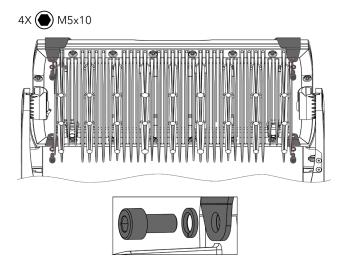
Secure accessory by 4 screws with spring washer at the back side of luminaire's head.
