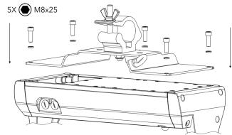
Mount the adaptor using 5 screws.
