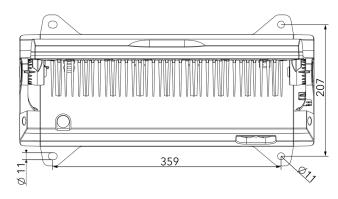
Drill holes to the surface according to holes spacing. Mount Divine via mounting holes on the surface.
