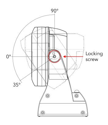
Release locking screw on each sides. Angle fixture to desired position and tighten locking screw on each sides.
