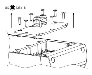
Inlets for power and data from side of the luminaire.
