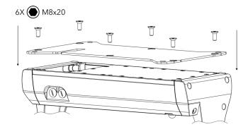
Mount the adaptor using 6 mounting screws.
