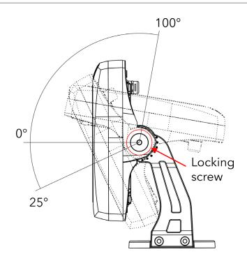
Release locking screw on each sides. Angle fixture to desired position and tighten locking screw on each sides.
