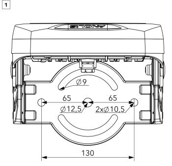
Drill 2 holes to the surface according to brackets spacing.
