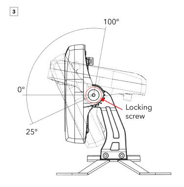
Release locking screw on each side. Angle fixture to desired position and tighten locking screw on each sides.
