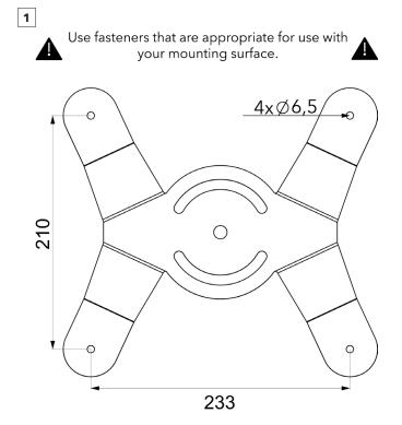
Drill 4 holes to the surface according to brackets spacing.
