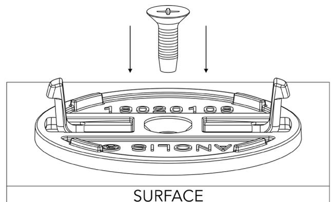
Take care not to over tighten the fastener to avoid damaging the mounting adapter.
