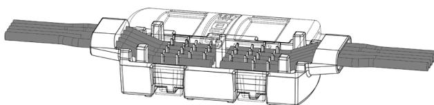
The cable cores are pressed by the cover and pushed to the contacts in base.
