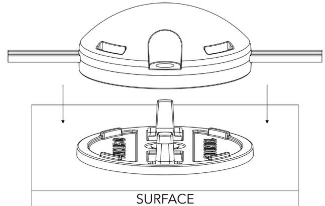
Every ArcPix II has an identification label with arrow on the bottom side. When you do your installation, keep the same orientation of the ArcPix II lines to ensure the same light characteristic of each line.
