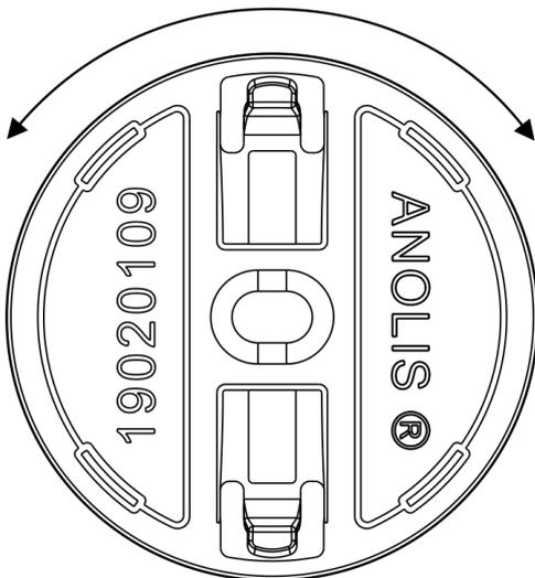
Prepare the correct mounting position of the adapter, making sure that all of them are oriented in the same direction.
