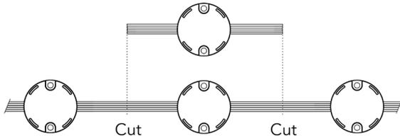
Cut away the faulty ArcPix II (carefully check the length of the new ArcPix II cable).
