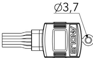
The hole in the housing of the termination box serves for screwing to the mounting surface.
