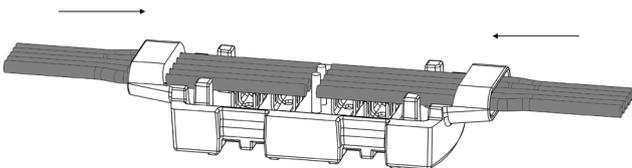
Separate cores in length 40 mm on the end of 5-wire flat cable. Insert cable trough the bushing into base of the connection box until it touches the partition in the connection box and align the cores into cutting edges.
