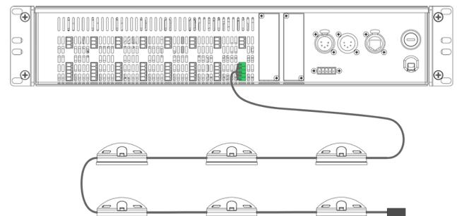
Connect ArcPixes to the LED outputs of the ArcPixel Power.
