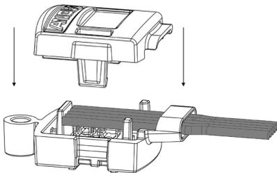
Put the cover on the base and press both parts together until both plastic catches snap into slots in the base of the termination box. For pressing use suitable plier with flat jaws if necessary.
