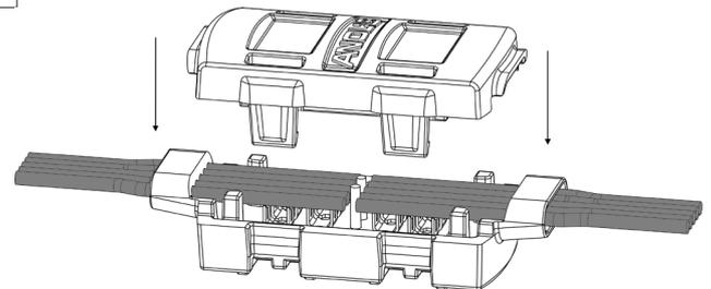
Put the cover on the base and press both parts together until four plastic catches snap into slots in the base of the termination box. For pressing use suitable plier with flat jaws if necessary.
