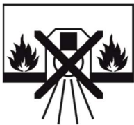
Suitable for fastening on non-flammable surfaces only
