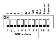
DIP 10 - if it is switched to ON=test light (the fixture lights at 3200K (for RGBW and TW version))
