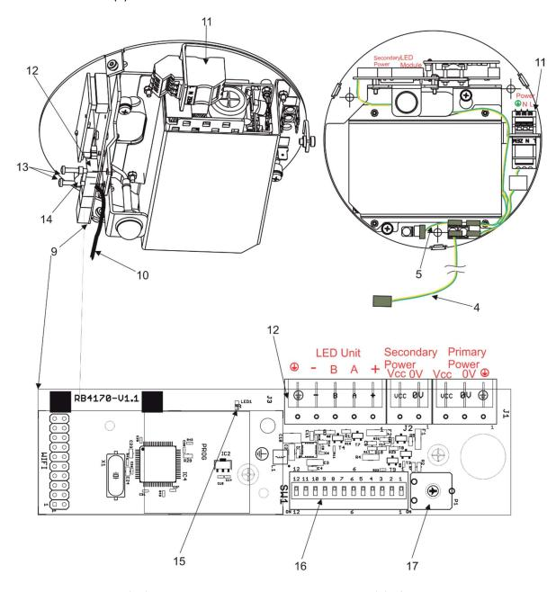
7. Pull the LED unit cable (10) through the bushing in the bottom cover (3) of the supply unit and connect it to the terminal block (12) and secure it by means of the clamp (14) and two screws (13).
