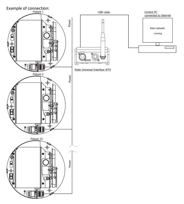
The fixtures have to be connected to power. The control PC should be connected to the Internet.
