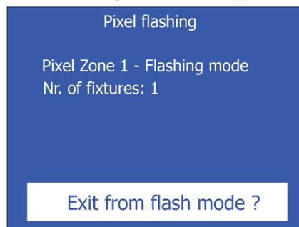
Now the ArcPower Unit Pixel is in the flashing mode. If you use the Robe Universal Interface, download corresponding update files for pixel modules (e.g. DSU\_ArcDot\_XXXXXXXXX.zip for ArcDots, DSU\_ArcPix\_XXXXXXXXX.zip for ArcPixes) from Robe web site at <https://www.robe.cz>. and continue as at FirmWareUpdate of the DRS via the Robe Universal Interface.
