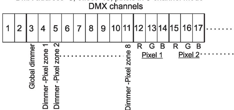
**Pixel Control** - the menu allows you to select a way of control pixel modules.
