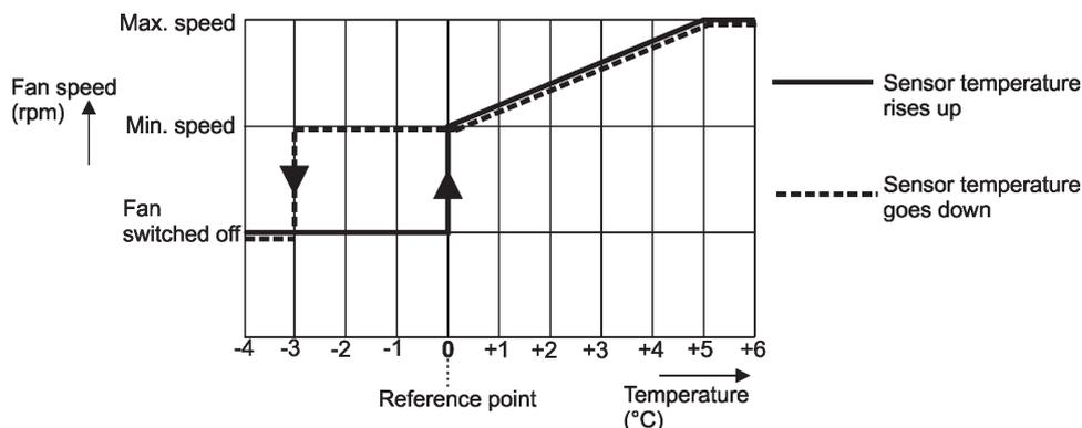
E.g. If a temperature in the Fan1 Threshold menu is set at 40°C, the controlled fan will behave as follows:
