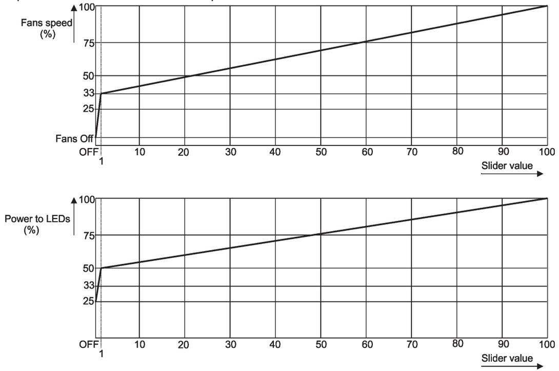
E.g. If the slider is set at 60, fans will operate in the range min. revs - 75% max. revs depend on current load.
