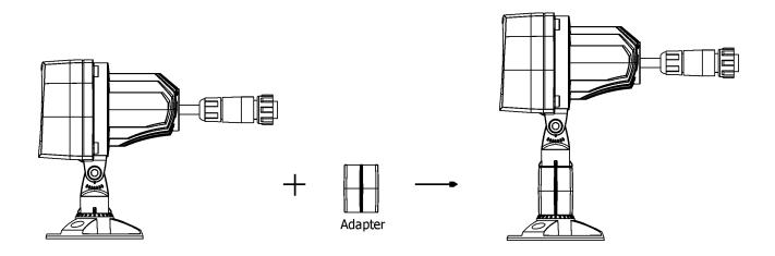
Use the following way for connecting of the ArcSource Outdoor 4 MC Pixel only (examples for matrix of 4x4):
