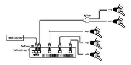
ArcSource unit is supplied with 1.5 m of cable for direct connection to the ArcPower drivers.
