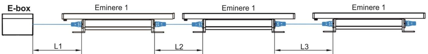
**Notice for the E-box Star:** The tables above state max. total number of Emineres connected to 6 Eminere outputs of the E-box Star (or max. number of Emineres connected to one Eminere output if the rest of Eminere outputs is not connected). The E-box Star has only one power input!
