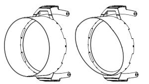
Unscrew the four socket head screws 6x10 (1) in Arc-Source Outdoor 24 MC housing and slide the top hat (2) onto ArcSource outdoor 24 MC and secure it with four socket head screws 6x10 through holes (3) in the top head.
