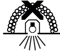
Unsuitable for covering by heat insulation material
