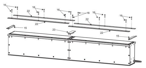
Note: If the Emineres Inground are installed in a loose soil (e.g. sand, gravel) the cover plate support (25) has to be fastened under the cover plate at outer (end) Eminere Inground. Screw the cover plate support (25) on the outside of the Eminere Inground by means of two screws Allen bolts M5x10 with washers and nuts M5.
