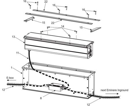
The supply/data cable to and from the mounting sleeve must be placed in a protective tube (12).
