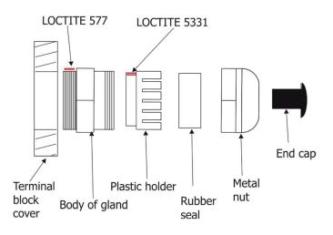
The cable gland M20 MS with a standard seal serves for a cable of diameter of 7-13mm, for smaller diameter of cable (4-8mm) you have to remove the original seal from the cable gland M20 and use the enclosed reducing seal instead of it. The reducing seal for diameter of cable 4-8mm (P/N 13051388) is enclosed in the Booster box.
