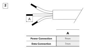
Strip these lengths for cable connections.
