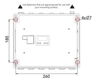
Drill holes to the surface according to holes spacing. Mount E-box via mounting holes on the surface.
